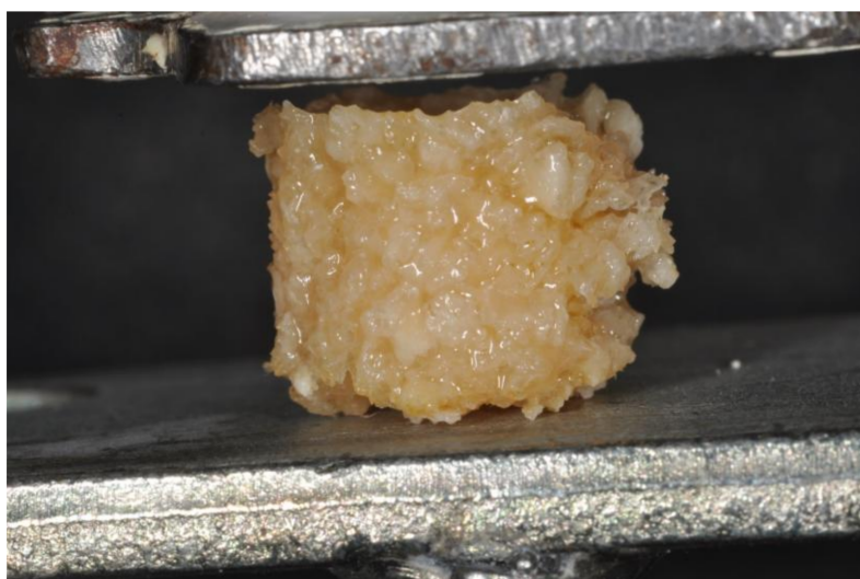
Figure 2. A cylinder of bovine bone mixed together with APL during the compressive test.
